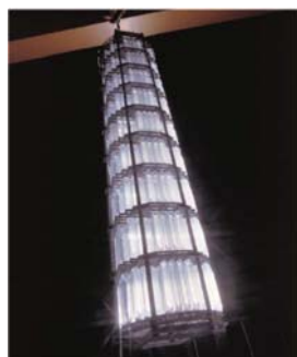
Artificial quartz crystal drawn from an autoclave
